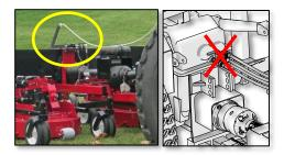
only two hydraulic hoses are required to run between the tractor and the mower. When the wings need to be raised or lowered, the operator simply uses the pull rope from the tractor's seat, which also releases the mechanical wing locks. The new **AUTOMATIC WING CYLINDER LOCK VALVE** makes operating the **Pro-Flex 120B** easier than ever before! For older mowers, an update kit (p/n 600600) is available.
